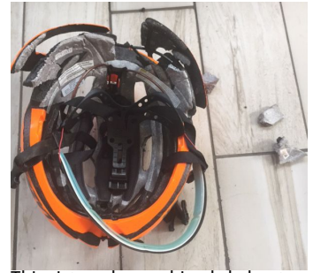
This picture shows a bicycle helmet that was damaged when a rider hit his head during a fall.
